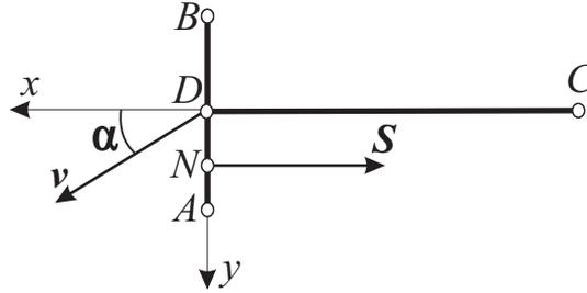
**Figure 2.** Plane-parallel motion of the free symmetric rigid body in a resisting medium
